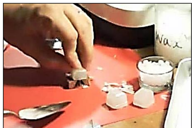
Figure 4. Fixing wax block to wooden chuck
